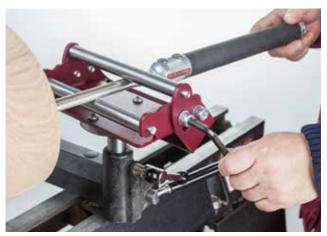
Slacken the cantilever locking screws and adjust the upper roller until it sits securely on the top of the tool shaft and lock into position
